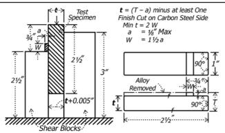
Shear Blocks shall be Bolted Firmly Together against Filler Piece which Provide Space 0.005" Wider than **t** of Specimen
